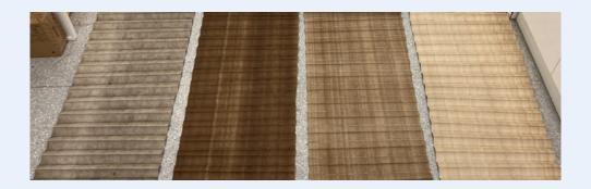
The 10-micron filter they were using was mainly removing particulate on the second layer. The upstream layer was too open so wasn't capturing much particulate. The second layer had too high an efficiency which was causing the filter to block.
